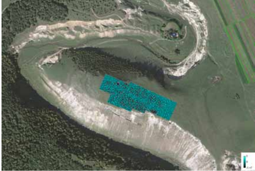
Fig. 4. Gordinești II- Stînca goală , Dist. Edineț. Magnetic map in the range of -5/5 nT in the colour scale imposed on the satellite image. The highest values are highlighted
