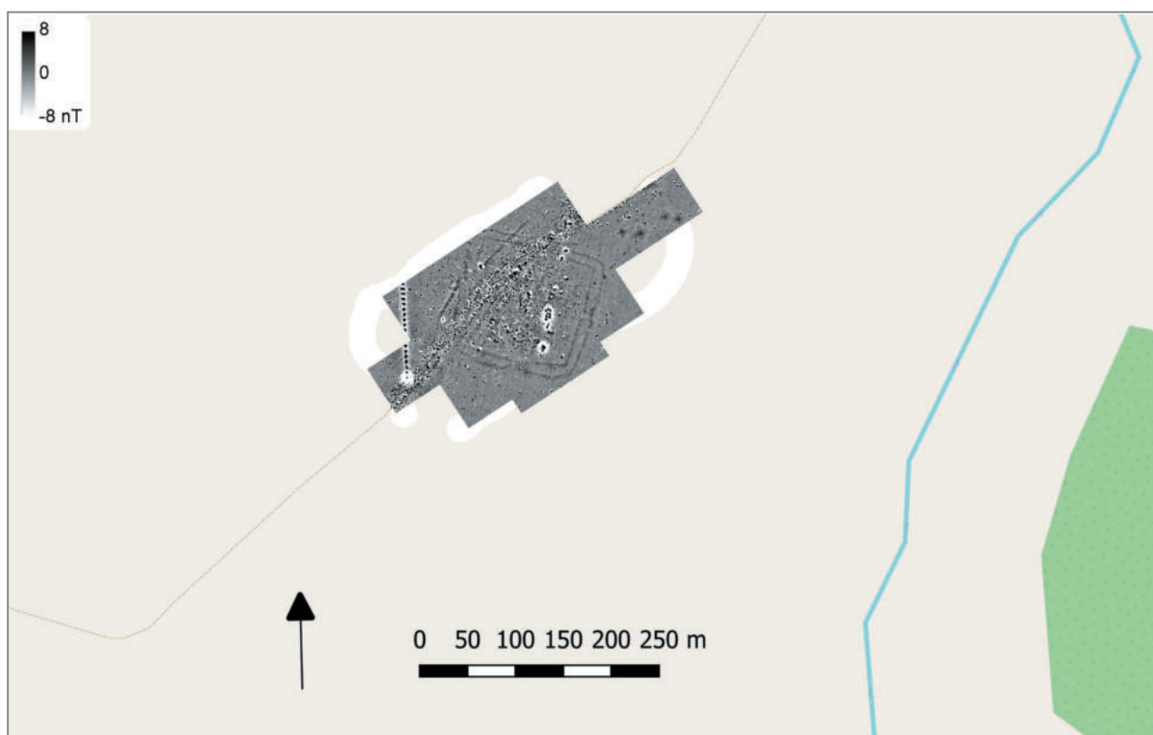
Fig. 11. Taraclia I. Magnetic map in greyscale, in range -8/8 nT, superimposed on the topographic map.
