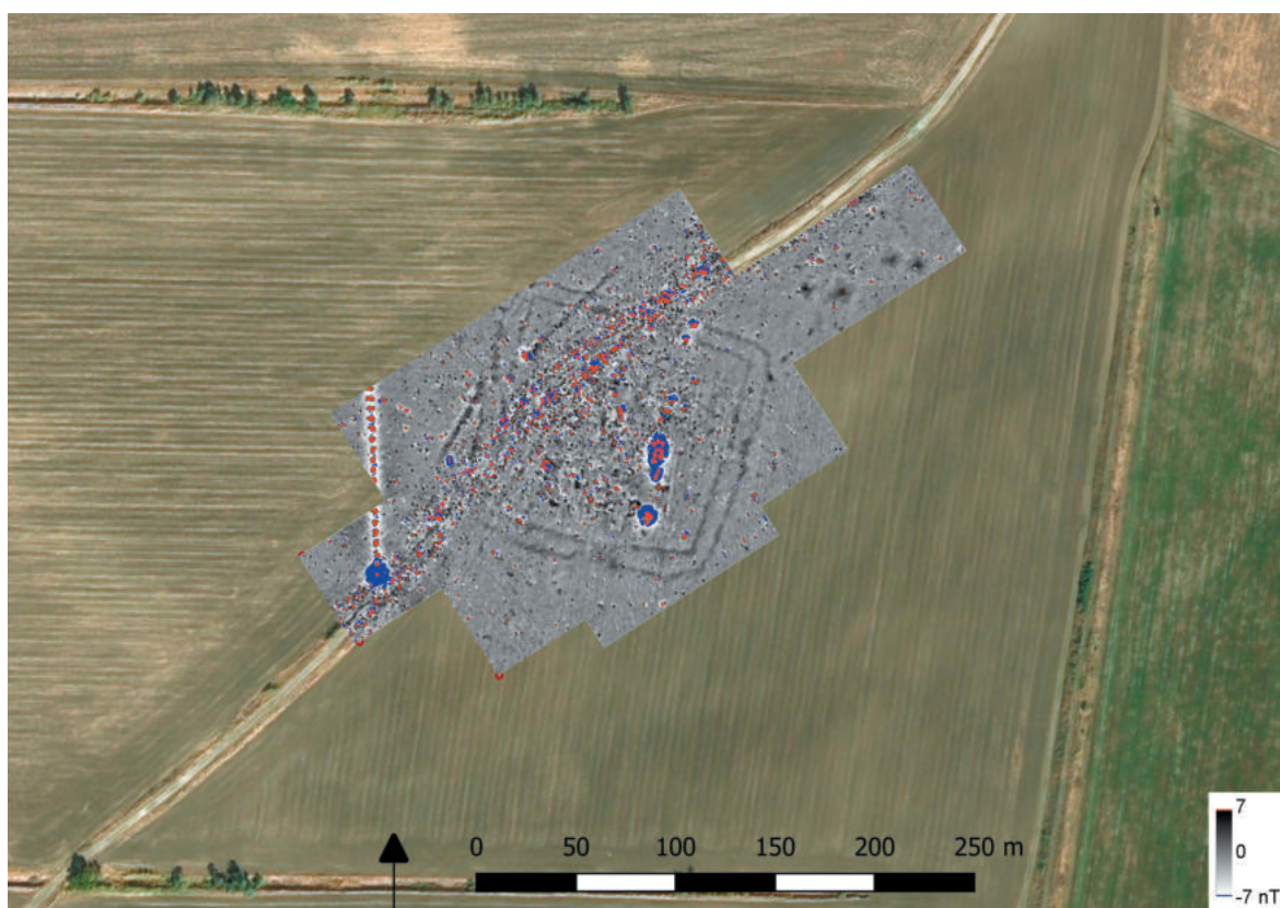
Fig. 13. Taraclia I. Magnetic map in greyscale with selected extreme values, in range -7/7 nT, superimposed on the ortophotographic map.
