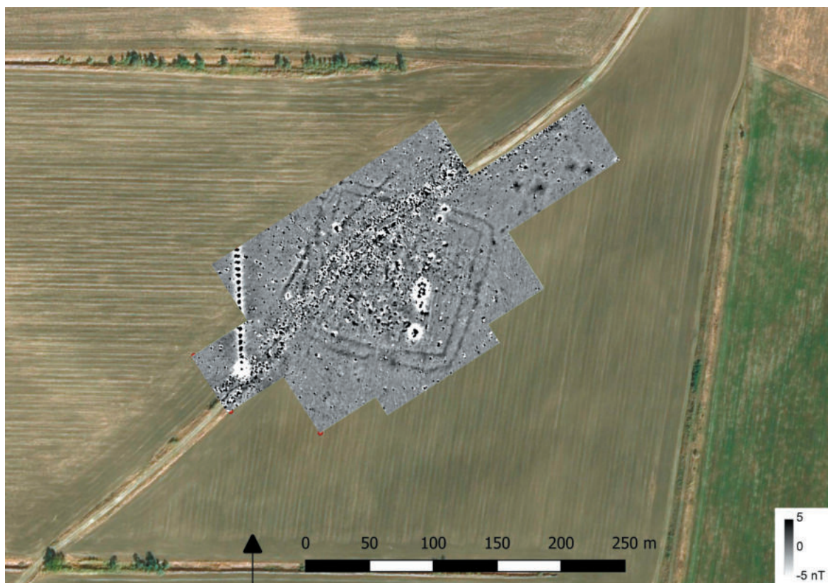
Fig. 12. Taraclia I. Magnetic map in greyscale, in range -5/5 nT, superimposed on the ortophotographic map.
