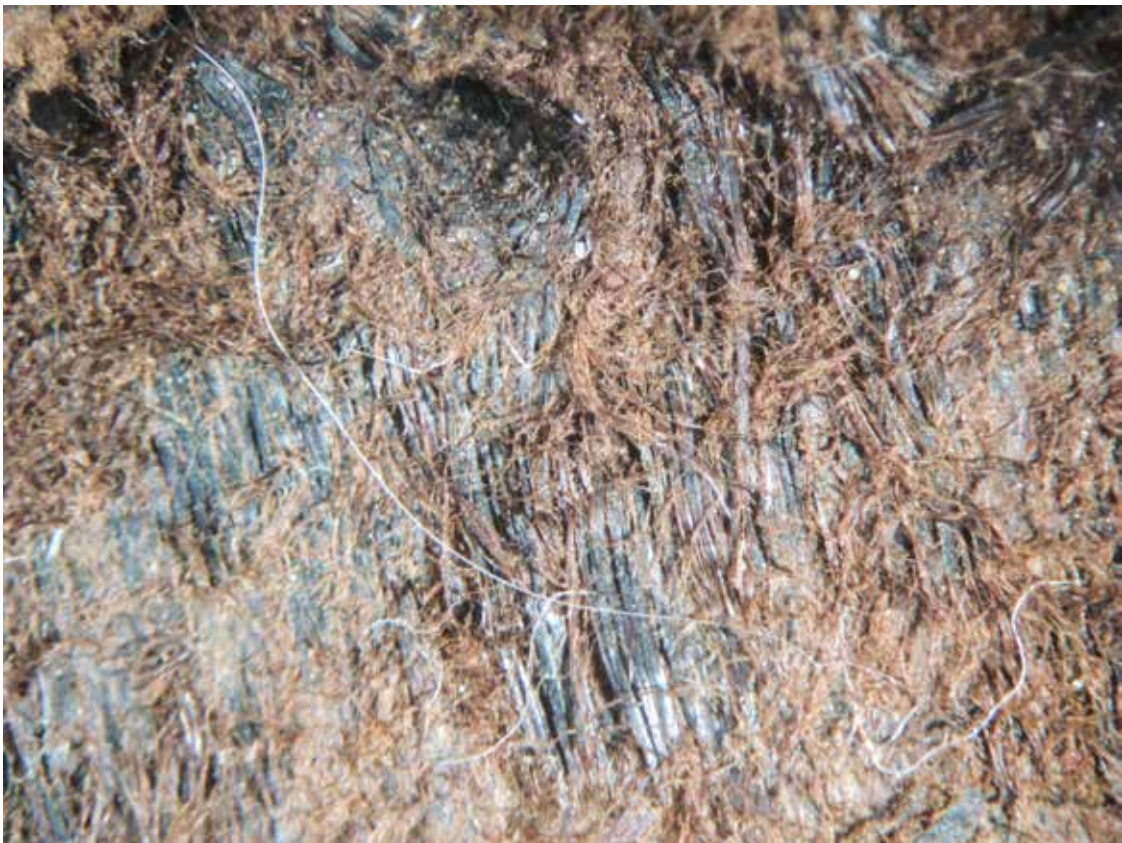
Fig. 6. Layer of subcutaneous tissues not removed during tanning – inner sole (photo by D. Grupa)
