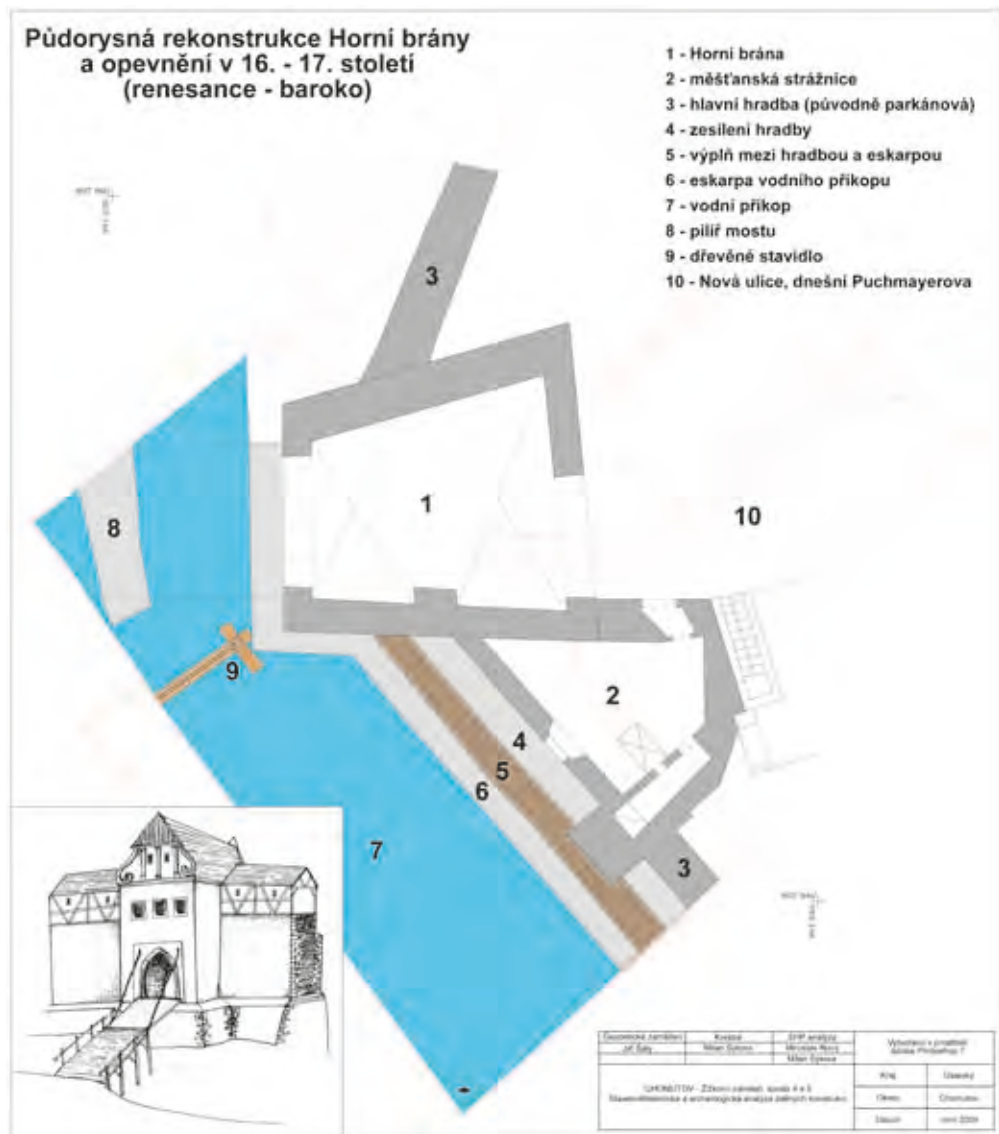
Fig. 17. Reconstruction of the outline of the Upper gate and the defensive walls in the sixteenth and seventeenth centuries on the basis of archaeological and archival research. 1 – the Upper gate, 2 – the townspeople watchtower, 3 – the main walls (originally inter-walls), 4 the thickening of the main walls, 5 – the space between the walls and the moat slope, 6 – the slope of the wet moat, 7 – the wet moat, 8 – the wooden bridge pillar, 9 – the wooden water gate, 10 – Nowa Street (now Puchmayerova) (drawing and interpretation by M. Nový – M. Sýkora)
