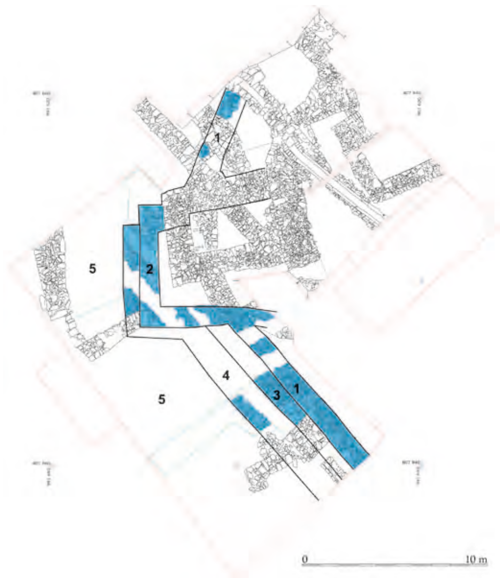
Fig. 16. Archaeologically researched fortifications of the western corner with the remains of the Upper gate. 1 – new main walls, rebuilt original inter-walls, 2 – the foundations of the Upper gate, 3 – thickening of the main defensive wall, 4 – the slope of the wet moat, 5 – the wet moat (drawing and interpretation by M. Nový and M. Sýkora)
