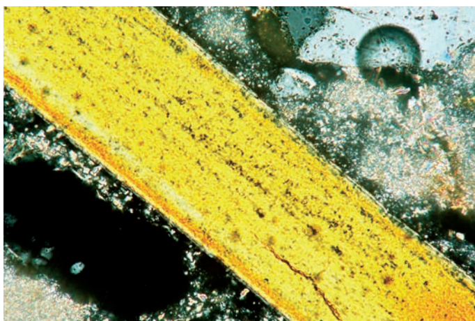
Fig. 12. 14 th century mortar from Czudec Castle. Fragment of a microorganism, filled with secondary iron compounds. Crossed polars, magn. x 400. Phot. M. Doktor.
