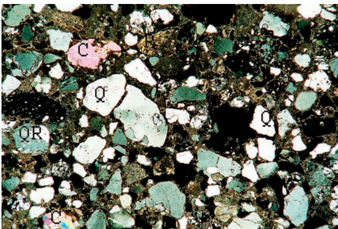
Fig. 1. 14 th century mortar from the ruins of Czudec Castle. Filler grains are composed of quartz (Q), calcite (C), fragments of quartz rocks (QR), fragments of other rocks (R). Black areas are caverns, pores and cracks. Filler grains are rounded in various degree, they may be grouped in two fractions: around 0.2 mm and around 0.5 mm and coarser. Crossed polars, magn. x 25, Phot. M. Doktor.
