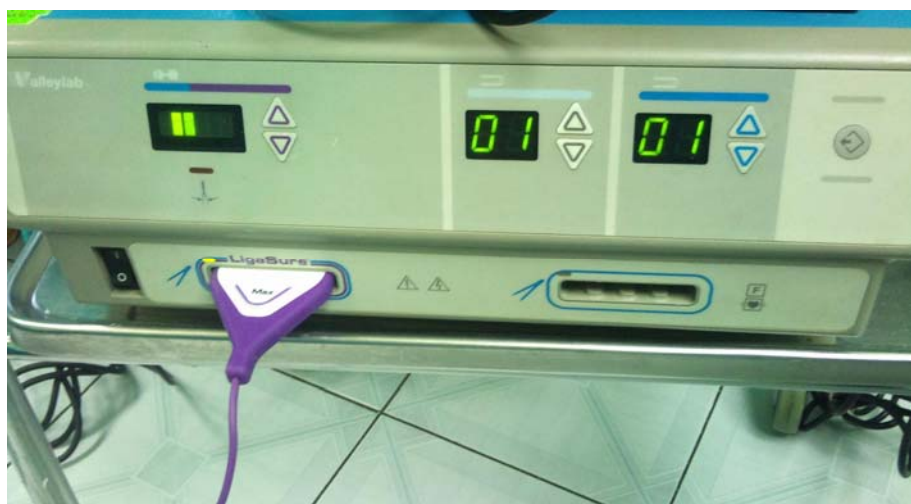
RYC. 1. Bipolarny system do zamykania naczyń LigaSure® - generator FIG. 1. LigaSure® bipolar vessel sealing system - generator
