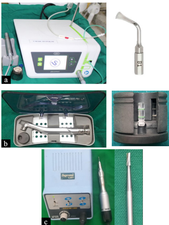
Fig. 3. A: WandH piezomed with B1 tip, B: Waterlase – iPlus (Turbo Mx7 handpiece with a spot diameter of 700 µm), C: Low-Speed Handpiece with 702 carbide bur
