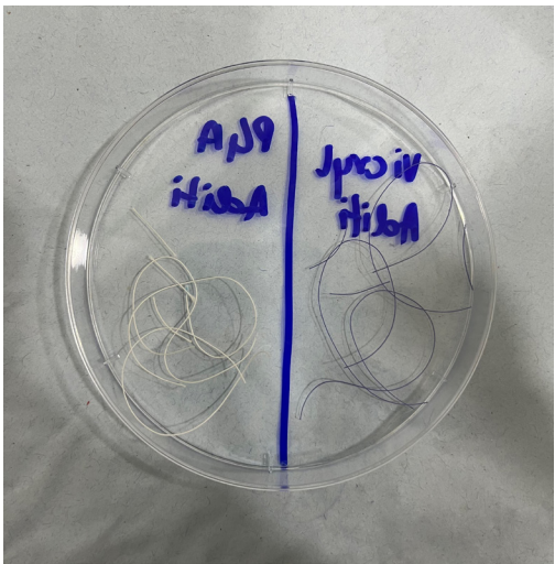
Fig. 4. Showing the air drying of the suture materials post immersion
