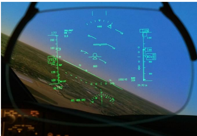
Fig. 6. Composite information displayed by HUD in aeroplane
