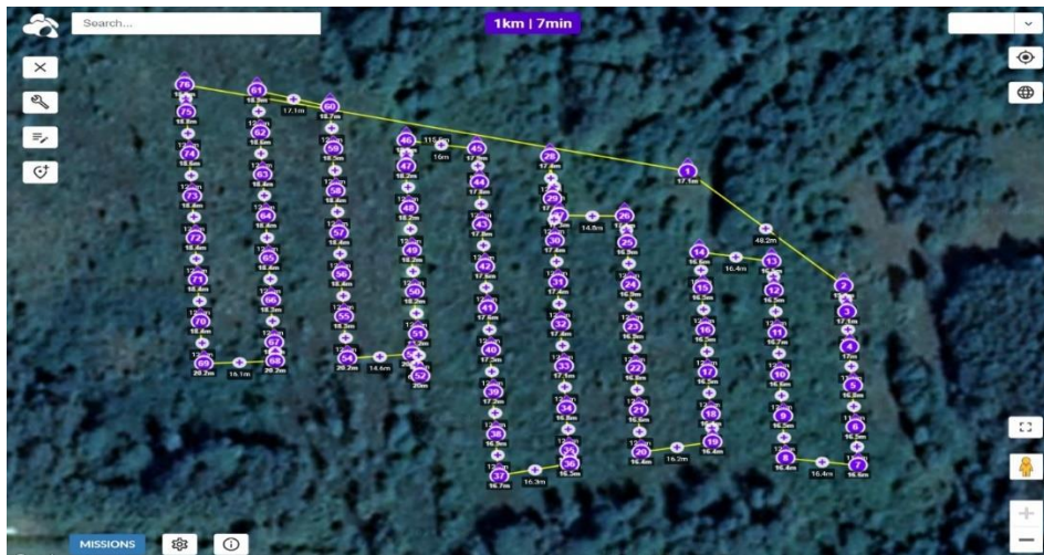
Fig. 1. Drone flight plan - screenshot of Litchi Mission Hub software Rys. 1. Plan lotu drona - zrzut ekranu z oprogramowania Litchi Mission Hub
