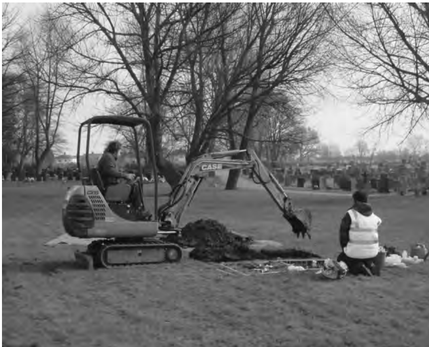
Fig. 1. Excavation of trench in Preston Cemetery beside area where Lumbricus terrestris burrows have been located and cast with coloured polyurethane resin
